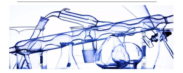
Glassware used in laboratories is unique in that it must be corrosion resistant, heat resistant and easy to handle. For these reasons, the majority of WINSON glassware is made from borosilicate glass.
