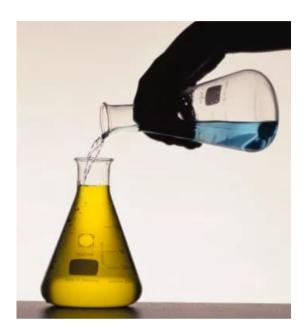
The Erlenmeyer Flask, an icon in the chemistry laboratory, boasts a conical design and a slender neck, ideal for holding, clamping, or sealing with a stopper. It's a versatile tool, adept in measuring, mixing, and storing liquids, with its unique shape lending stability and reducing spill risk.
