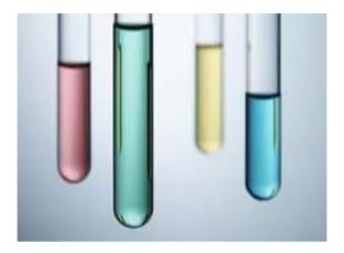
A test tube, the quintessential symbol of scientific inquiry, is a cylindrical vessel of resilience. Typically shaped with a round bottom, these tubes are masterfully crafted from borosilicate glass, a material renowned for withstanding temperature fluctuations and resisting chemical reactions.
